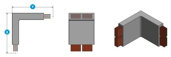
Standard **X** & **Y** = 350mm, Min. **X** & **Y** = 300mm, Max. **X** & **Y** = 1000mm
