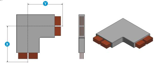
Single Construction - Copper 1000A to 3200A, Aluminium 800A to 2500A Standard & Y = 350mm, Min. & Y = 300mm, Max. & Y = 1000mm
