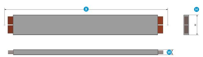
Standard lengths = 3m, 2m & 1m. Min.  $\chi$  = 0.5m, Max.  $\chi$  = 3m.  $\psi$  = 90/100/120/140mm
