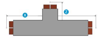
Standard X = 1000mm, Min. X = 700mm, Max. X = 1500mm Standard / Min. Z = 300mm, Max. Z = 750mm
